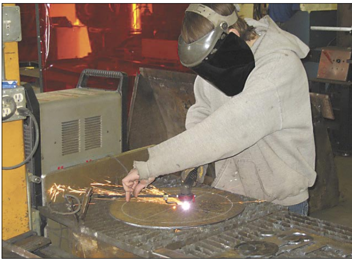
Juniors’ work benefits public works Top: Jonathan Verwer of Homedale, left, and Jake Black of Parma stand behind some of the water meter covers they recently fabricated inside Mark Bauer’s COSSA welding shop in Homedale. Middle: Black stands watch as Verwer guides the arm of a Computer Numerical Controlled plasma cutter over a slab of black iron to cut out a disc that would be come a meter. Above: Once the meter cover is cut, Black does additional work. Submitted photos
